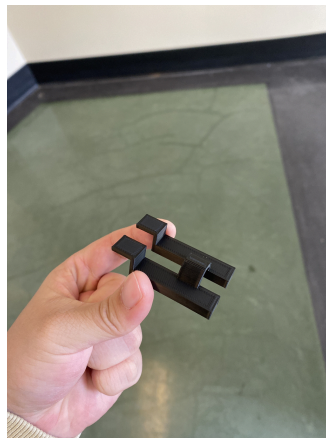
Figure 13. Printed IR laser holder
